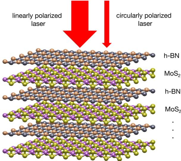
FIG. 3. A layered van der Waals heterostructure to realize the dielectric tensor of Eq. (2) for the case of  $\epsilon_{xy} = -\epsilon_{yx}$ . The linearly polarized laser shining on the heterostructure provides uniform gain for both valleys of MoS<sub>2</sub> while the circularly polarized laser provides a small, additional gain for only one valley.
